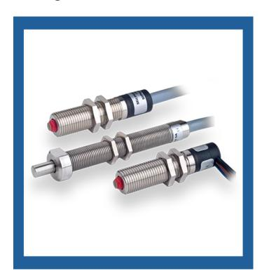
The High Precision Limit Switches (MP600) are designed with a long-life sensing mechanism to detect two positions with a few microns of accuracy and a high degree of repeatability within a single, compact cylindrical body. Depending on the cable choice, they can operate on a temperature range from -40°C to 130°C. The cable can be supplied with a connector termination, typically M8 or M12.
