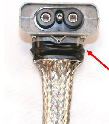
A shielded sleeve can be used to surround un-shielded cable.
