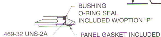
CUTAWAY ILLUSTRATION OF PANEL SEAL DRESS RING
